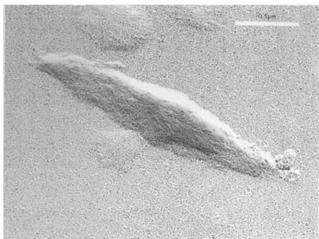
Figure 6 TEM micrograph of a Ryton V-1 PPS big crystal grown at T_c = 201^\circ\text{C} and T_c = 175^\circ\text{C}
